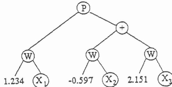
Figure 4: Representation of a neural network as a LISP expression. 'W' represents a multiplication operation by an input weight and 'P' represents a summation and the node nonlinearity.
