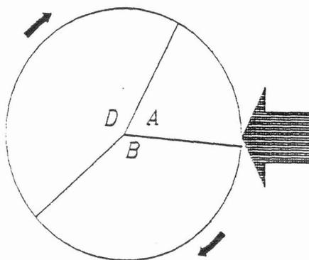
Figure 1: Selection. Units are selected for reproduction with probability proportional to their fitness. Units with higher fitness (corresponding to more slots on the roulette wheel) are more likely to be chosen than units with lower fitness, but all units have some chance of being chosen.
