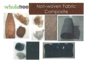
Figure 7. Creation of a trunk lid by substituting coir for polyester in the non-woven fabric composite of polyester-polypropylene that is compression molded into various trunk trim parts.
