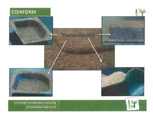
Figure 8. Excellent formability in compression molding of non-woven fabric composites with 50 wt% coir.
