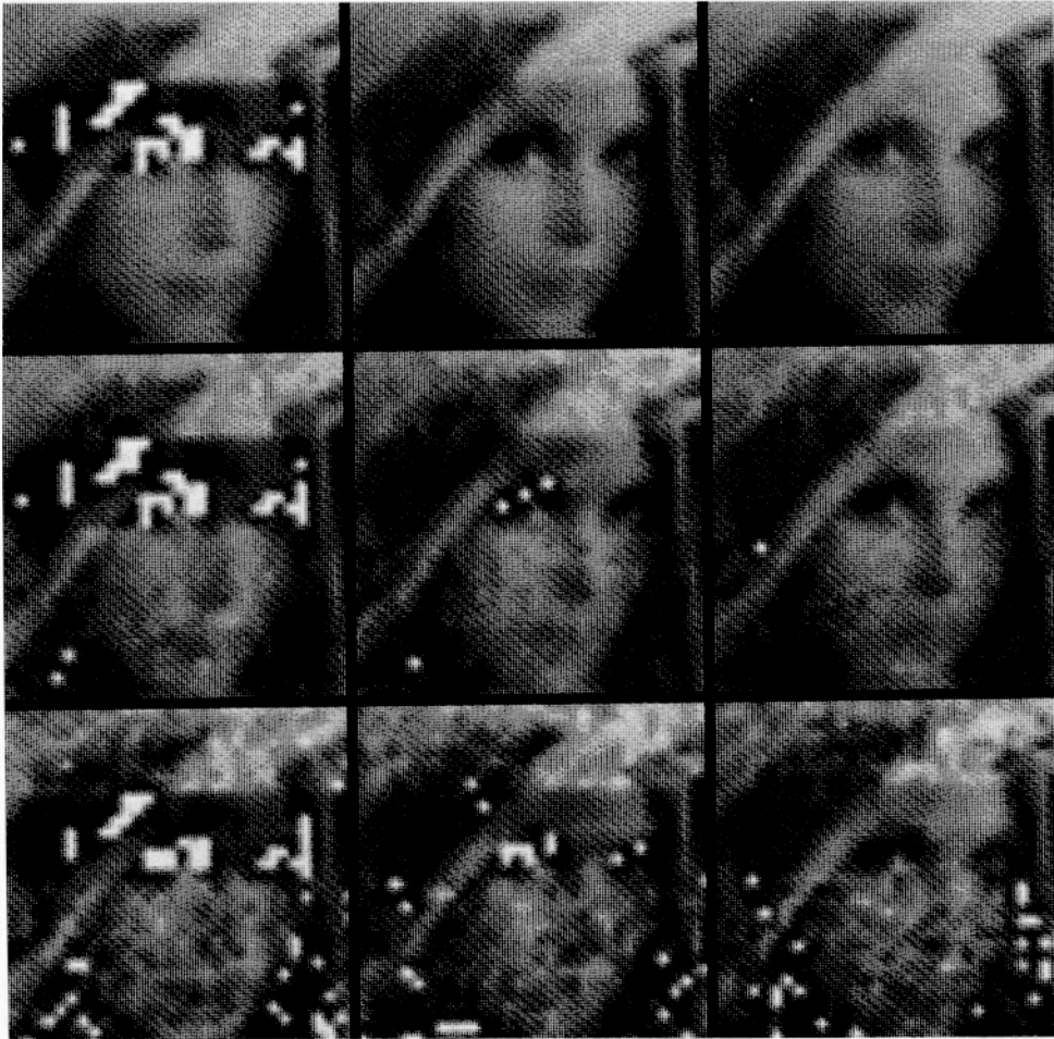
Fig. 8. Image reconstruction with static gaussian noise for 25% floating neurons. Here, and in the figure to follow noise is measured as the ratio's of the standard deviation to the full dynamic range of the gray level. The top row has 1% noise (iterations 0, 4, 10). The middle row has 5% noise (iterations 0, 5, 11). The bottom row has 10% noise (iterations 0, 5, 10).
