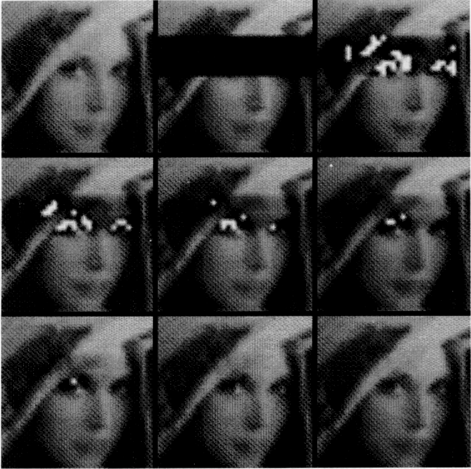
Fig. 1. Image reconstruction sequence. Top left to lower right sequence: original image, clamped image, iteration 0, iteration 1, iteration 2, iteration 3, iteration 5, iteration 10, iteration 19. A total of 40 images were stored on the APNN. Each image is 32 \times 32 .
