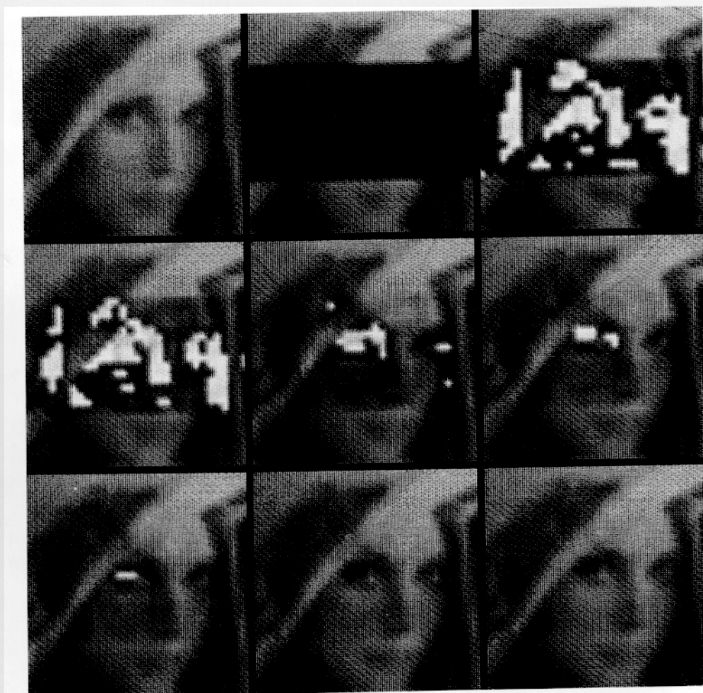
Fig. 3. Image reconstruction using the same net used in Fig. 1. Here, the percentage of clamped neurons is reduced to 75%. Top left to lower right sequence: original image, clamped image, iteration 0, iteration 2, iteration 20, iteration 40, iteration 60, iteration 80, iteration 101. Clearly, more iterations are required.
