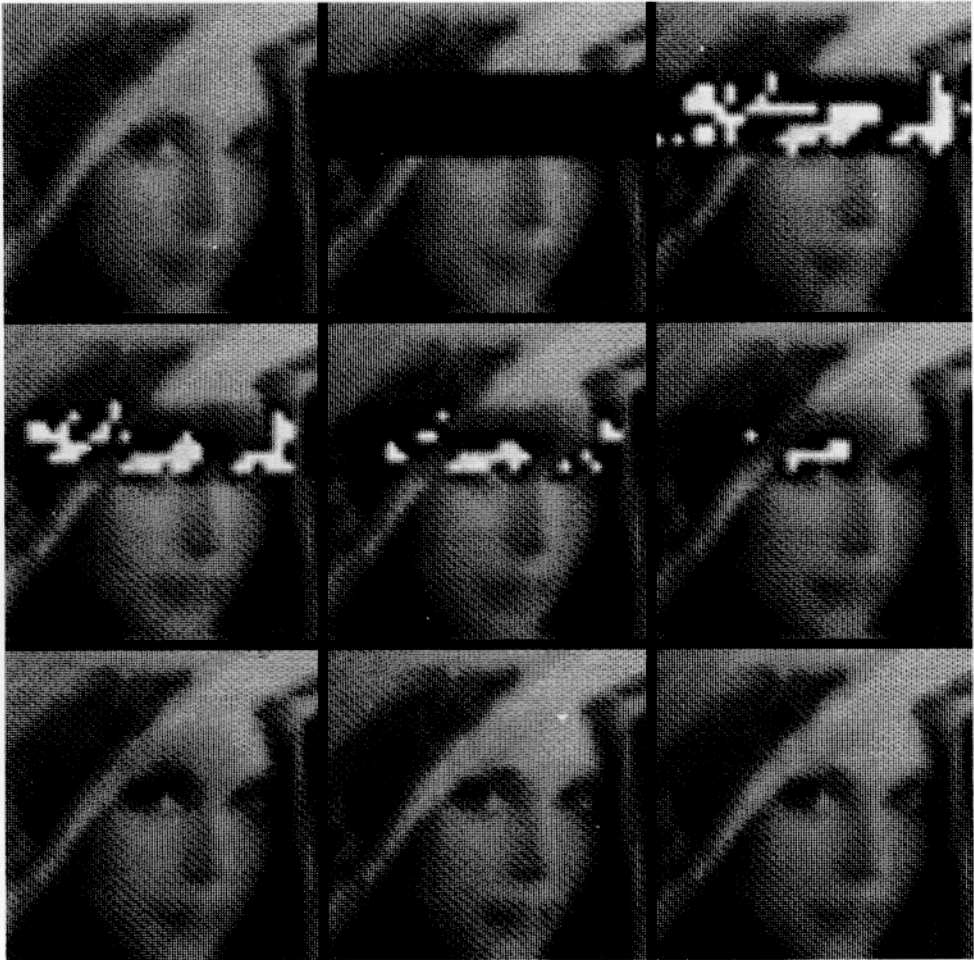
Fig. 4 . Image reconstruction sequence when the number of the library images is 160. Top left to lower right sequence: original image, clamped image, iteration 1, iteration 5, iteration 21, iteration 20, iteration 50, iteration 150, iteration 208. Comparing to Fig. 1 , convergence is slowed as more images are stored in the net.
